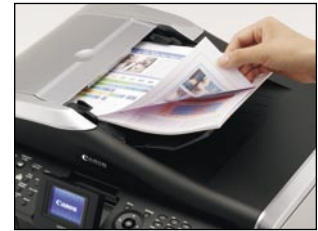
Auto Duplex ADF (MP830 only) for double-sided copying and scanning
